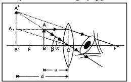
Magnifying power of a simple microscope is defined as the ratio of the angles subtended by the image and the object on the eye, when both are at the least distance of distinct vision from the eye.
