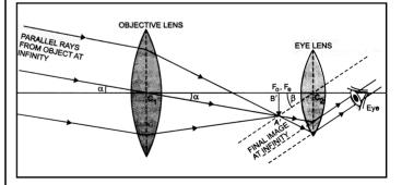
However, in astronomical telescope, final image being inverted with respect to the object does not matter, as the astronomical objects are usually spherical.
