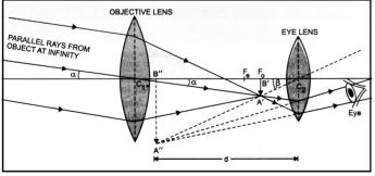
Magnifying power of an astronomical telescope is defined as the ratio of the angle subtended at the eye by the final image at the least distance of distinct vision to the angle subtended at the eye by the object at infinity, when seen directly.
