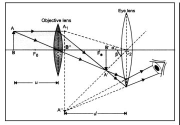
Magnifying power of a compound microscope is defined as the ratio of the angle subtended at the eye by the final image to the angle subtended at the eye by the object, when both the final image and the object are situated at the least distance of distinct vision from the eye.
